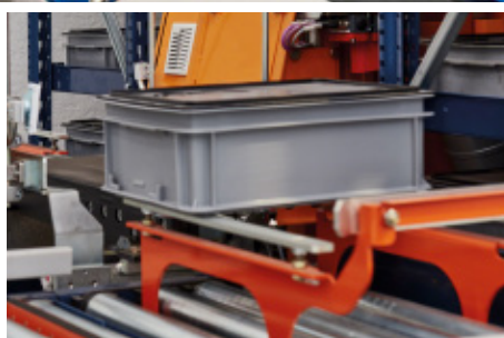
Roller conveyors with delayed lifting capabilities collect and drop off loads for the stacker crane at the front of the miniload system.
